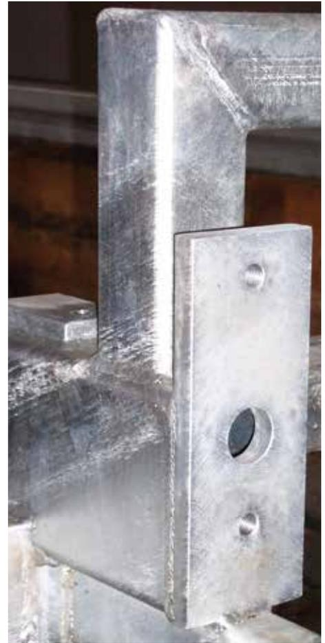
Machined Mounting Pads/Tubular Steel Frame
