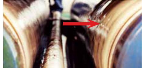
BDP's vertical arrangement eliminates the problem of filtrate running off upper rolls and pooling around lower rolls.
